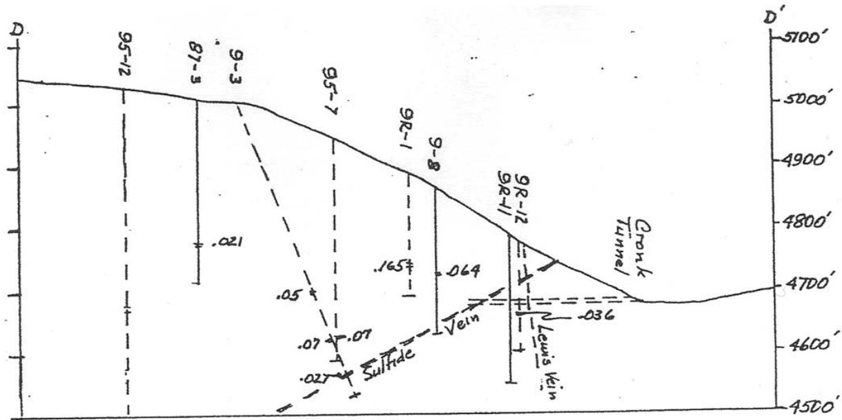
Figure 5. Cross section through the Cronk Tunnel looking northwest showing projections of the Lewis and Sulfide Veins.
