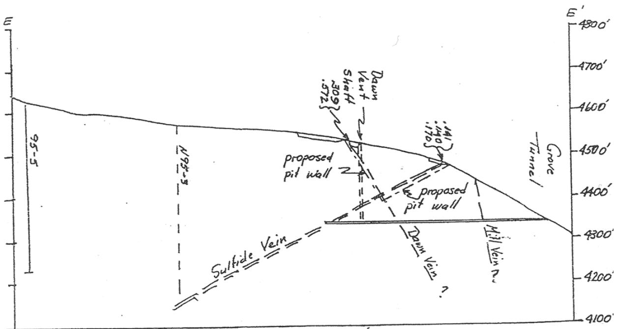
Figure 6. Cross section through the Dawn Area looking north-west showing projection of the Dawn shaft, the Grove Tunnel, the Dawn Vein, the Mill Vein, and the Sulfide Vein. The proposed open pit is also shown.
