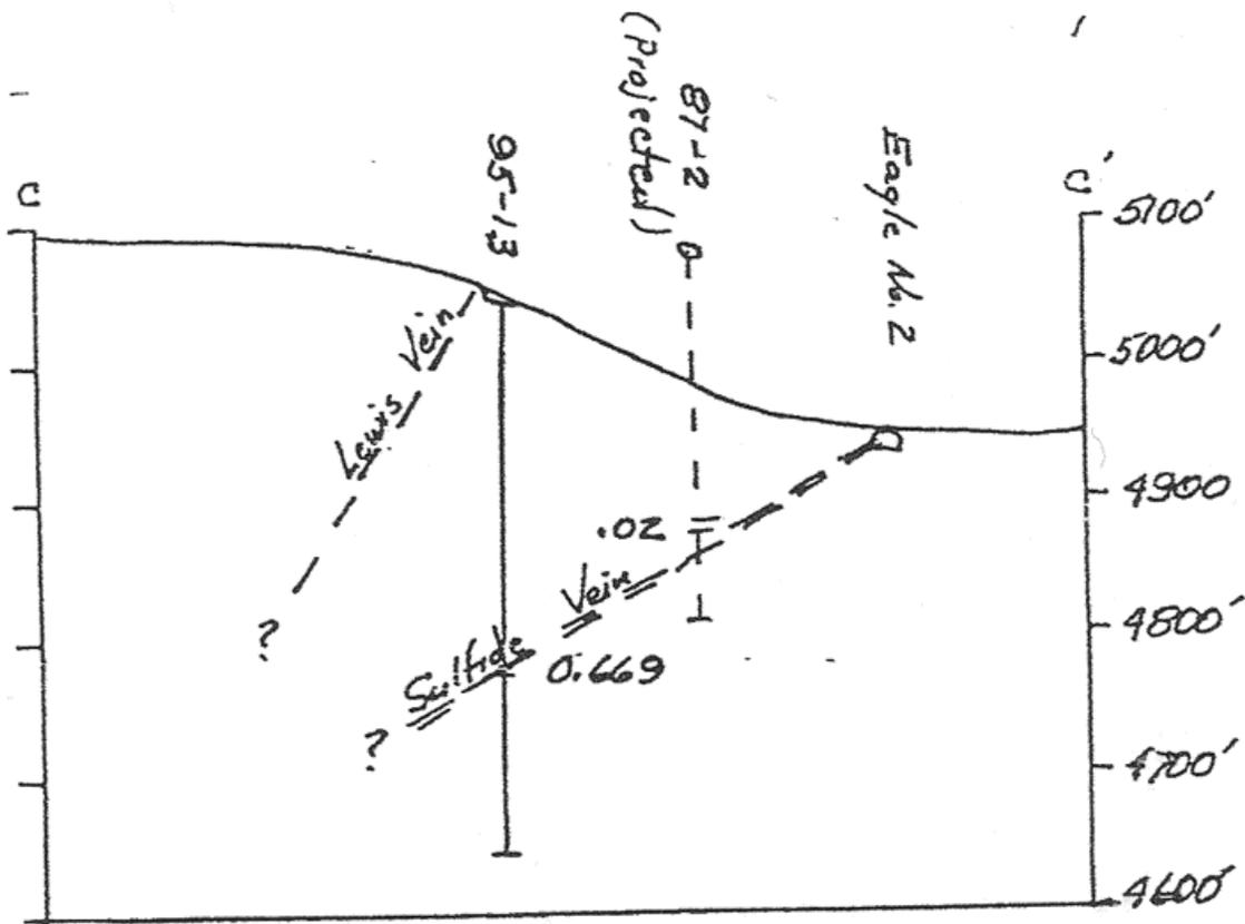
Figure 4. Cross section through drill hole 95-13 looking west showing the projection of the Sulfide and Lewis Veins.
