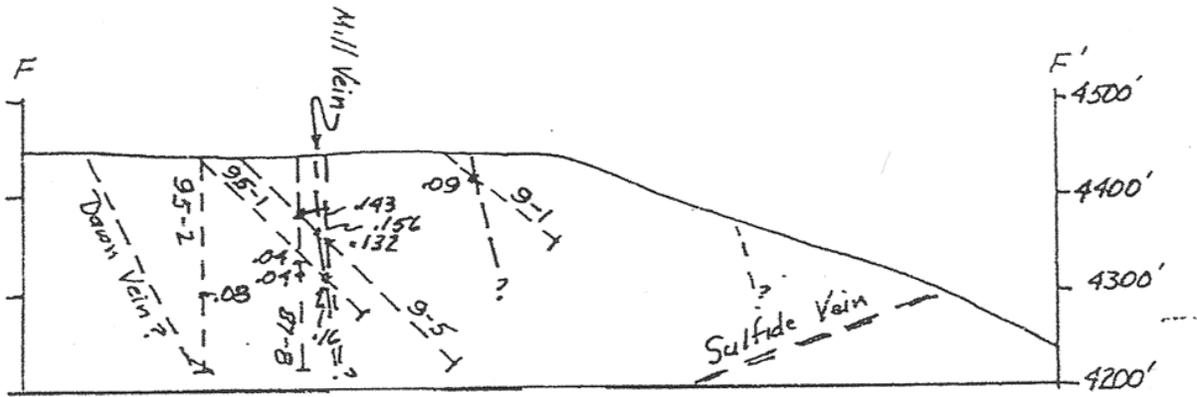
Figure 8. Cross section through the Protection Area looking northwest showing several drill holes projected to the plane of the section along with vein intercepts.
